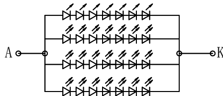
Backlight LED Circuit I_f=80\text{mA}; V_f=21 \pm 2.1\text{V}
